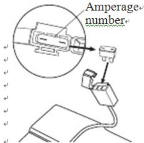
Remove the fuse and replace with a new one of equal amperage. Requires 30 amp fuse. Close the fuse cover and reattach the battery cover.
