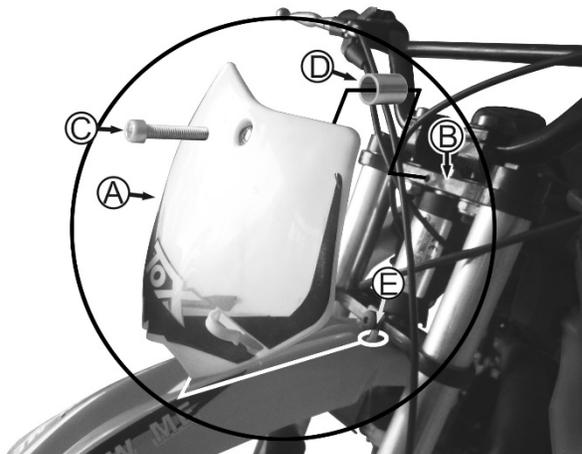
1. Insert the number plate (A) onto the two pegs on the front fender (E)
