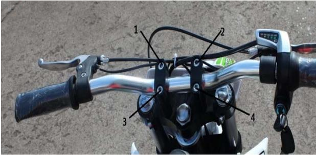
1. place the handlebar (A) in the bottom clamp, then cover the upper clamp (B) on the handlebar and install the 4pcs bolt (C)
