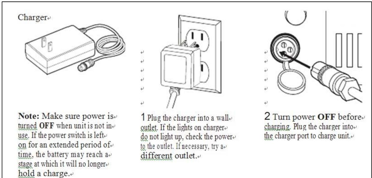
**Warning:** Failure to recharge the battery at least once a month may result in a battery that will no longer accept or hold a charge.
